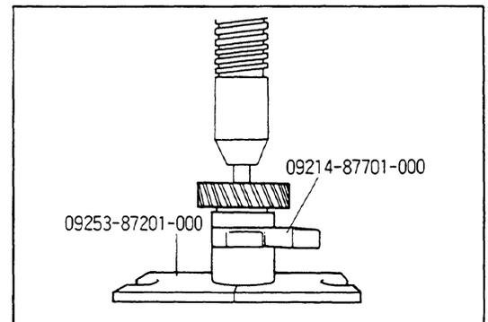
4. Replace the shaft's gear after the shaft has been refinished. Use special service tools # 09253-87201, 09506-87303, and 09214-87701.
