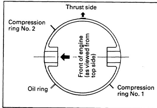
4. Insert the connecting rod and piston assembly into the cylinder block with a piston ring compressor attached.
