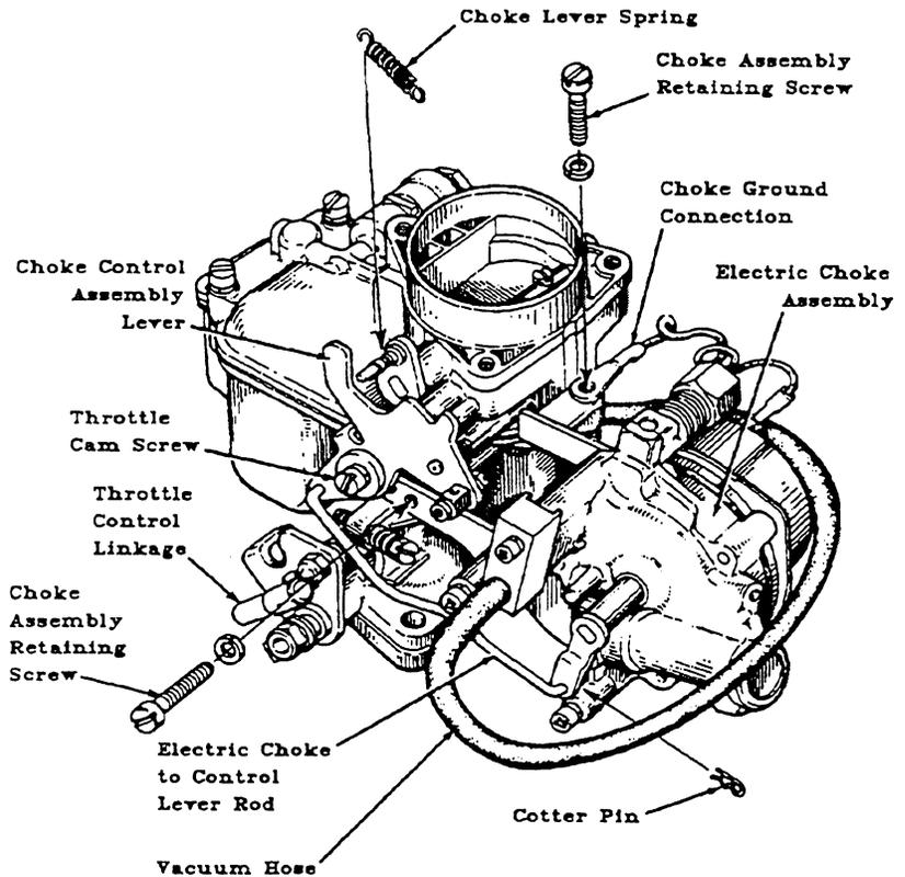
4. Remove the two choke assembly retaining screws and their washers. Disconnect the electric choke assembly from the carburetor.
