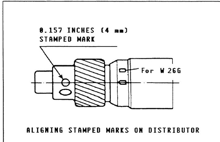
3. Install the distributor into the cylinder block in such a way that the mold seam line provided on the distributor body is lined up with the embossed line located on the distributor housing.
