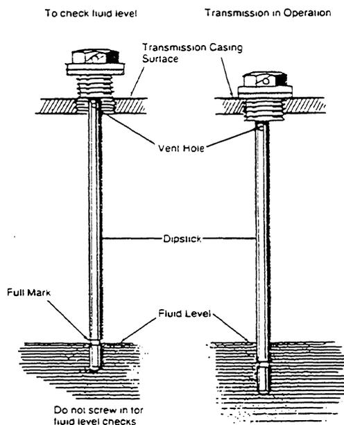
To check the fluid level, just insert the dipstick. Do not screw in. Retighten the hex screw with the dipstick after the fluid level check. Do not omit the O-ring seal.
