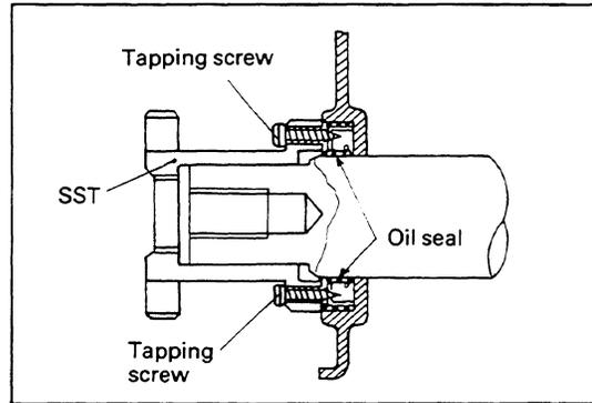
E. Remove the oil seal by extracting the oil seal remover tool with the puller (4).
