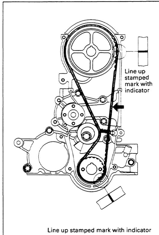
6. Rotate the crankshaft two complete turns in the normal direction of rotation until the No. 1 piston returns to Top Dead Center (TDC). Check that the timing belt pulleys again are properly aligned with their respective indicators, as indicated in step 5.
