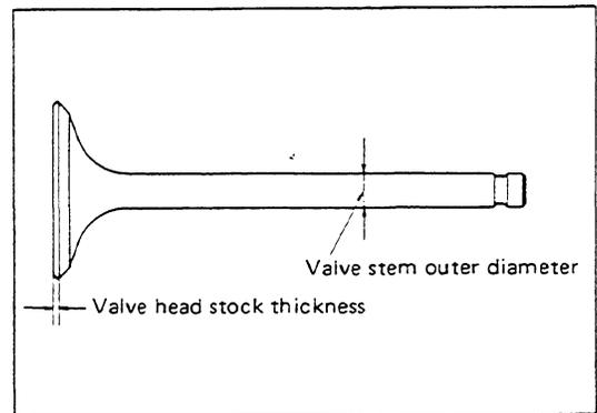
5. Check for excessive grooves at the end of the valve stem.
