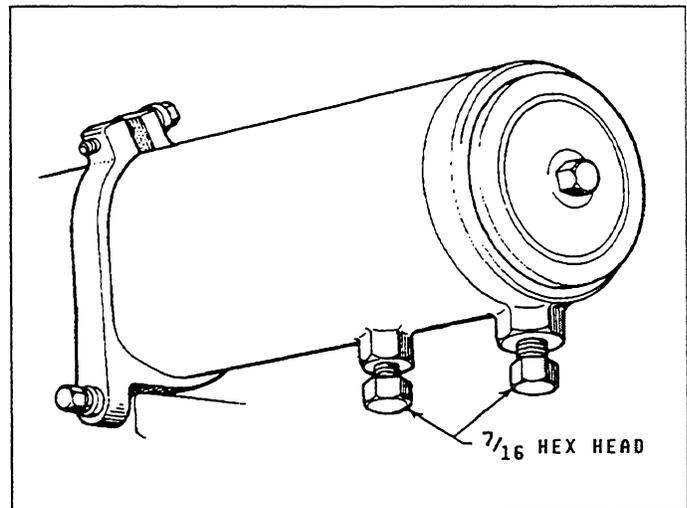
Heat Exchanger Drains
