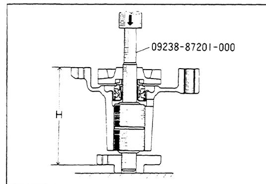
4. After the water pump has been assembled, make sure that the rotor rotates smoothly.
