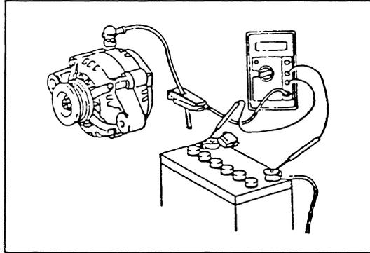
2. To test the stator, use an ohm meter to check the resistance between each terminal.
