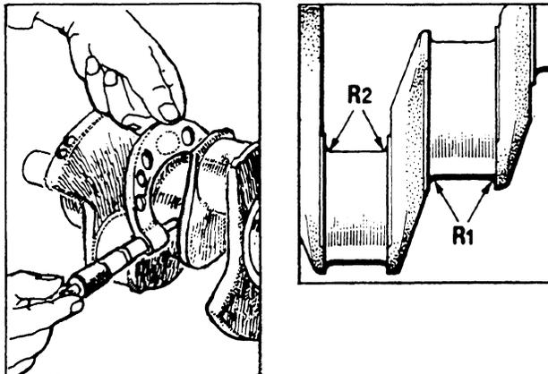
5. Measure the crankshaft's runout.
