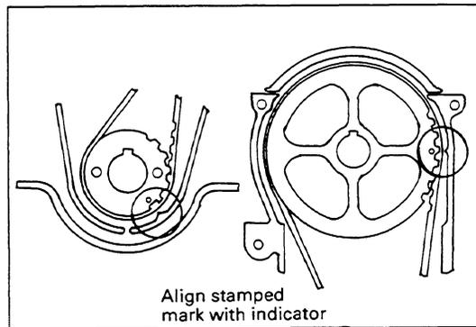
2. Temporarily attach the timing belt tensioner, leaving its setting bolt backed off one half turn.
