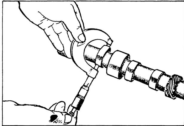
4. Measure the camshaft journal-to-cylinder head journal clearance. Replace the part that exhibits the most wear.
