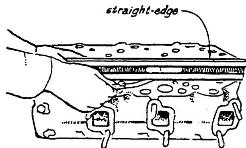
Specified Cylinder Head Height: 4.953 inches (125.8 mm)
