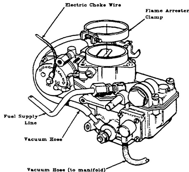
Carburetor with flame arrester removed.
