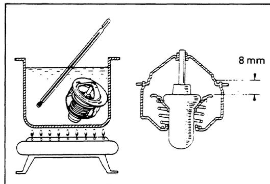
3. Replace the thermostat if the valve remains open at normal temperatures or if the valve is loose when the valve is fully closed.
