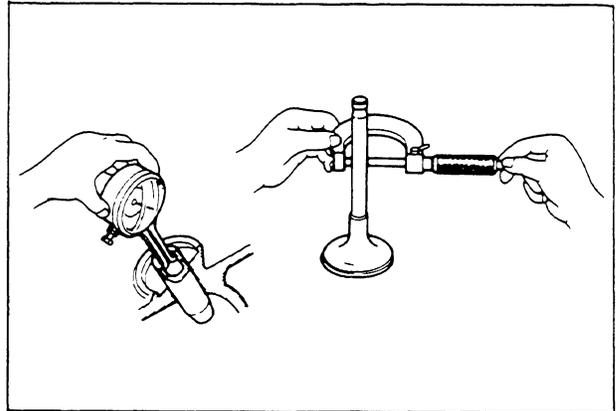
Measuring Method #2: Check each valve's deflection with a mounted dial indicator by moving the valve stem from side to side.
