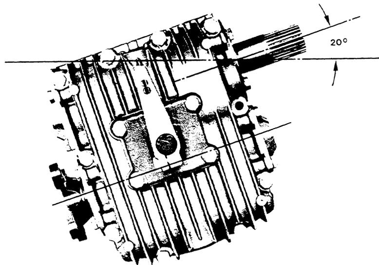
The position of the cover plate underneath the actuating lever is factory-adjusted to ensure equal lever travel from neutral to position A or B.
