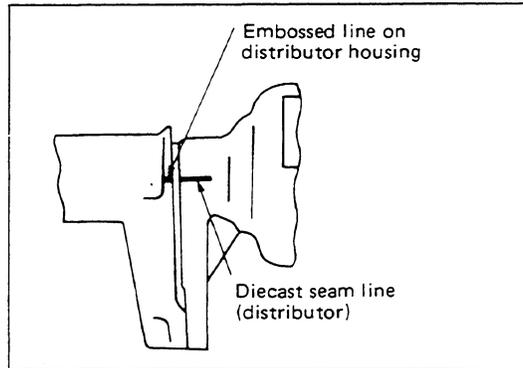
4. Temporarily tighten the distributor retaining bolt.
