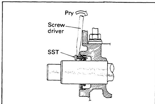
D. Align the oil remover tool in the punched hole (aligning it with the punch) and screw in the tapping screws to hold the oil seal remover tool.
