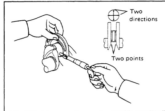
**NOTE:** Measure the diameter of each of the crankpins and main journals at two points (the front and rear portions) at 90 degrees to the crankshaft axis, as shown in the figure.
