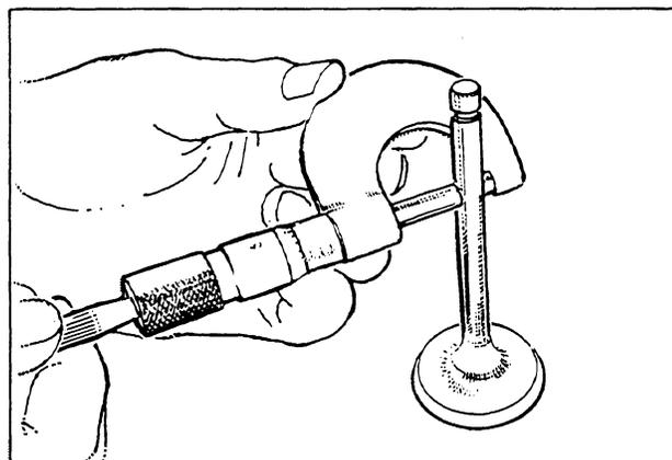
4. Check of each valve's head stock thickness. Replace the valve if it is beyond the allowable limit.
