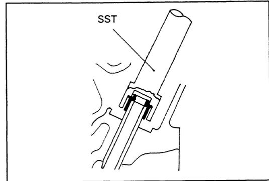
2. **NOTE:** For this step, temporarily insert the rocker arm shafts (see step# 4). Insert a valve, compress the valve springs, using special service tools # 09202-87001 and 09219-87702, and install the spring retainer locks. Repeat this process for each valve.
