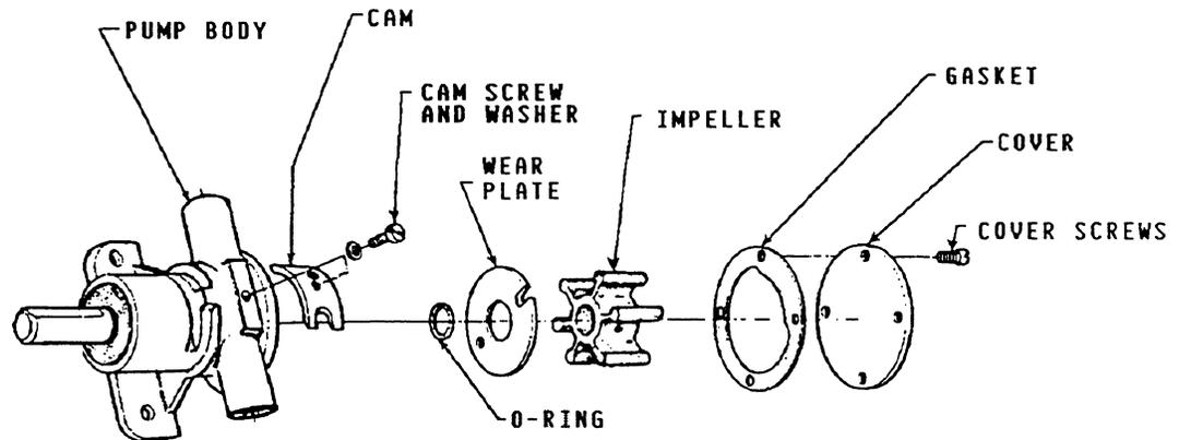
1. To disassemble the sea water pump, remove the four cover screws.
