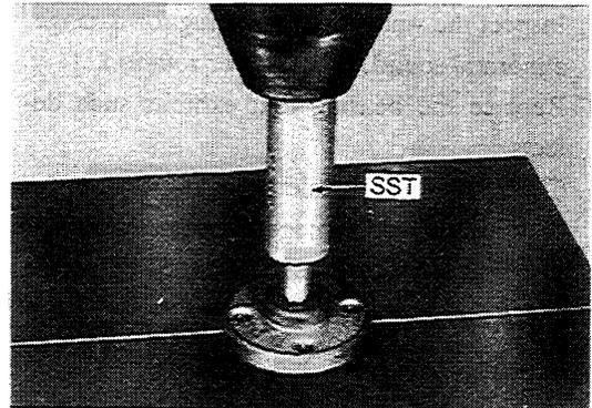
2. Using the same special service tools as in step #1, press off the water pump's bearing and seal set.
