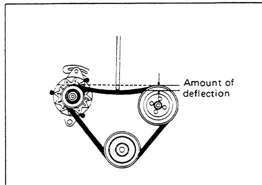
8. Install the sea water pump's mounting bracket and the sea water pump; install the drive belt and adjust the belt so that it deflects between 0.43 to 0.51 of an inch (11 to 13 mm).
