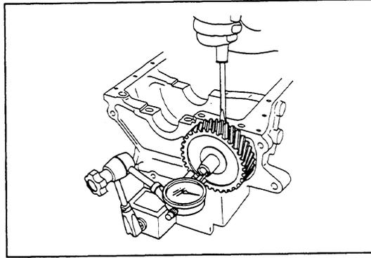
2. Measure the balance shaft's oil clearance.
