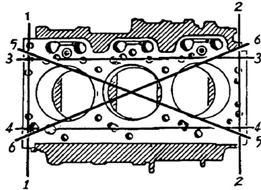
4. Check for scratches or burns on the cylinder walls. If necessary, repair by boring each cylinder or replace the cylinder block.
