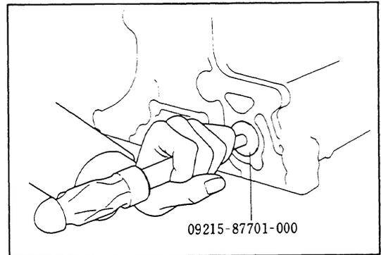
2. Install a new, or undersized bearing depending on the journal conditions, with the same special service tool used to remove the bearing.
