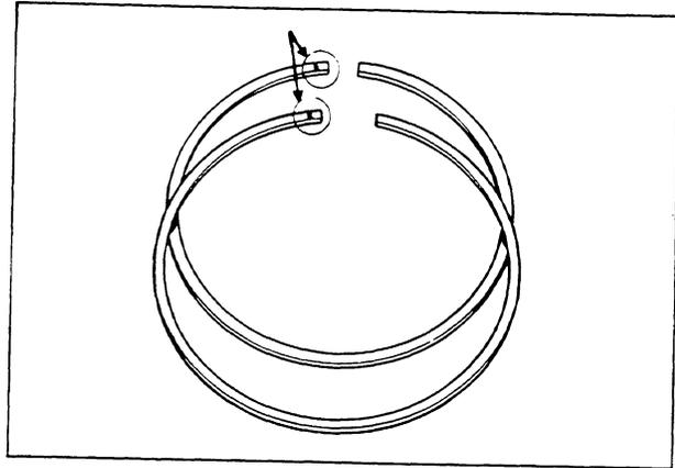
2. Make sure that the ring openings **DO NOT** align when they are on the piston. Position the ring gaps in the direction shown in the figure.
