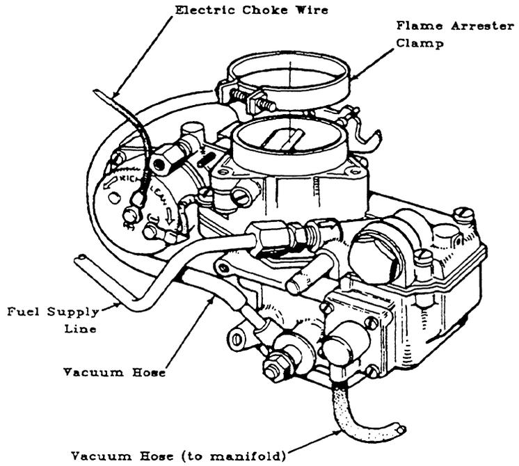
2. Remove the two nuts holding the carburetor to the manifold and lift the carburetor from the manifold.
