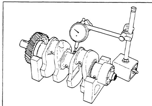
7. Check the crankshaft's thrust clearance with a feeler gauge, as shown in the figure. If it exceeds the allowable limit, replace the thrust washer.
