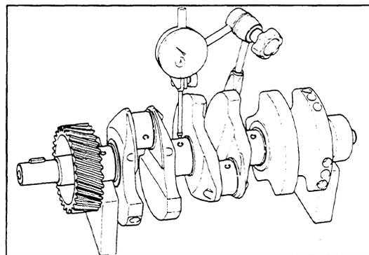
6. Measure the crankshaft for bend by placing a dial gauge at the center bearing journal and turning the crankshaft, as shown in the illustration to the right.
