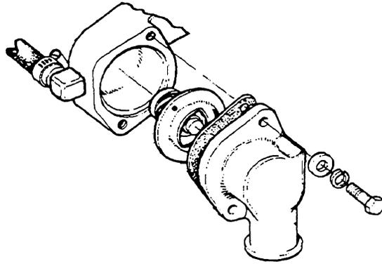
2. To test the thermostat, immerse it in water and gradually heat the water. The thermostat should start to open when the water temperature reaches 176 to 183° F (80 - 84° C). The thermostat should open by more than 0.31 inches (8 mm) when the water temperature reaches 203° F (95° C).
