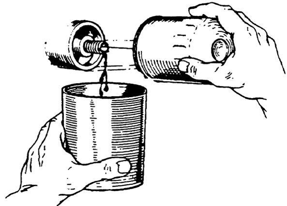
**NOTE:** Generic filters are not recommended, as the material standards or diameters of important items on generic parts might be entirely different from genuine parts. Immediately after an oil filter change and oil fill, run the engine to ensure that the oil pressure is normal and that there are no oil leaks around the new oil filter.
