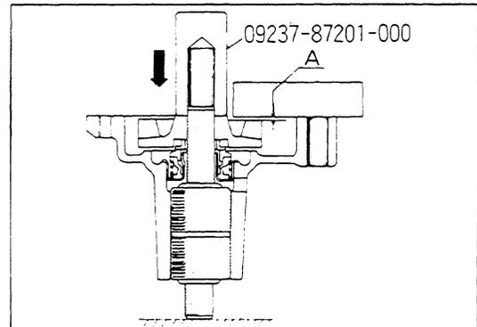
3. Press the water pump assembly into the water pump's pulley seat. Make sure that dimension **H** is maintained between 3.78 to 3.80 inches (96 - 97 mm)
